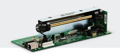
The Andros® 6500 and 6520 OEM gas modules achieve high reliability through simplicity of design and implementation. Andros Non-Dispersive Infrared (NDIR) gas modules are inherently reliable because there are no moving parts in the optical path. Unlike alternative analyzers that require motors, gratings, chopperwheels, and/or other moving components with limited useful lives, Andros gas analyzers use a pulsed infrared source to achieve high accuracy with high reliability.
